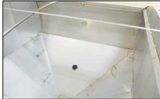
Fig 23 - Compartment ladder rungs
