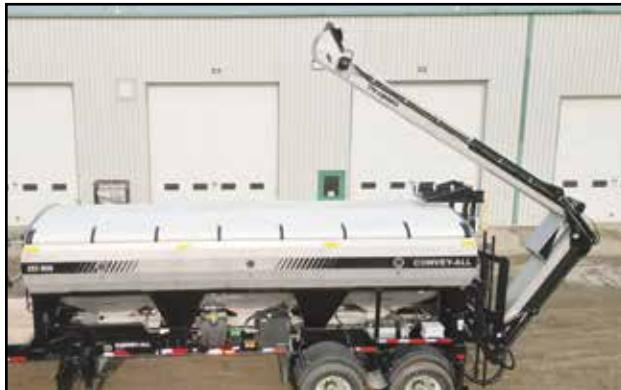
Fig 35 - Unfolding incline conveyor
