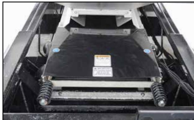
Fig 60 - Underbin conveyor tension bolt and springs
