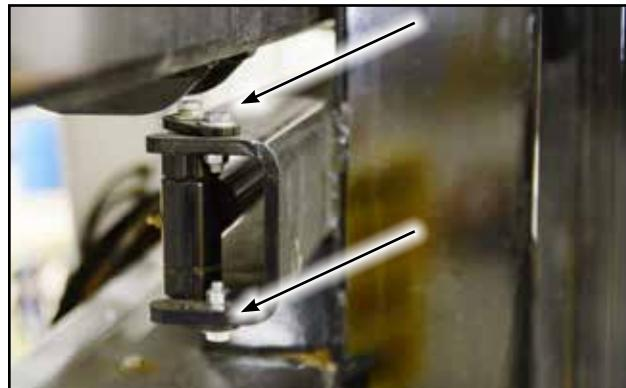
Fig 27 - Cylinder frame connection
