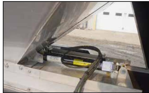
Fig 38 - Compartment discharge gate cylinder
