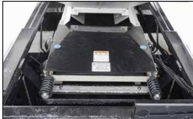
Fig 62 - Tension bolt on underbin conveyor
