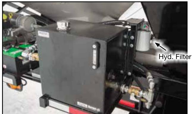
Fig 66 - Hydraulic oil reservoir and filter
