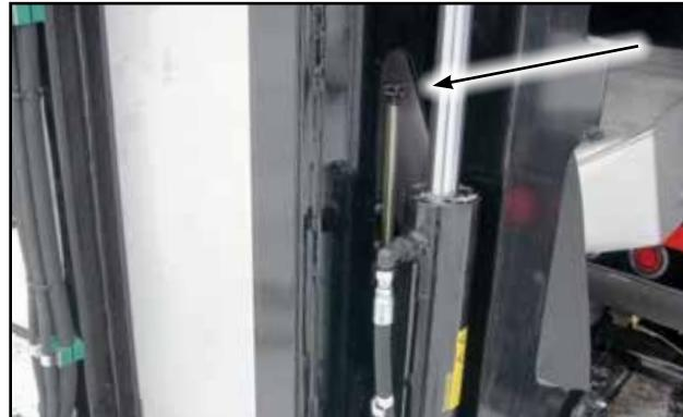
Fig 61 - Tension bolts on incline conveyor
