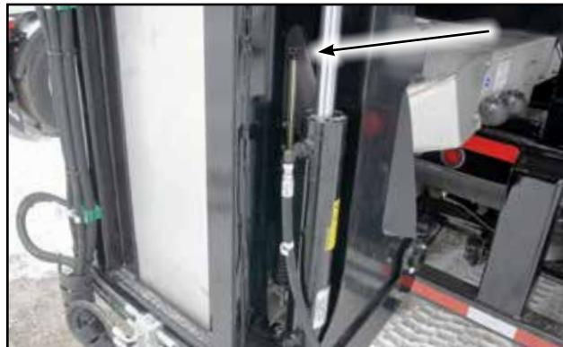
Fig 63 - Tension bolts on incline conveyor
