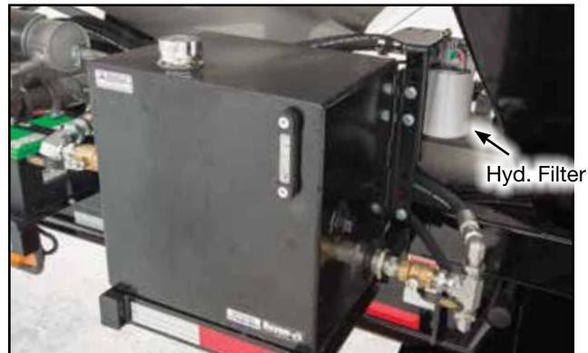
Fig 58 - Hydraulic system and filter
