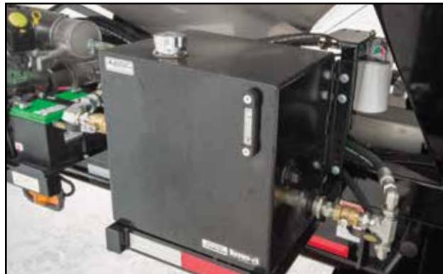
Fig 48 - Hydraulic oil reservoir
