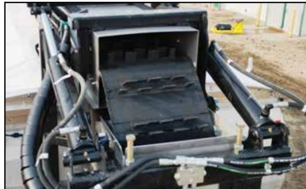
Fig 17 - Paddle belt on incline conveyor
