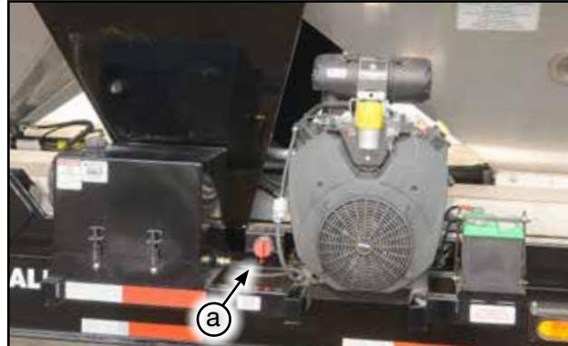
Fig 8 - Fuel tank, lock-out switch, engine and battery
