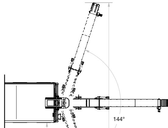
Fig 36 - Incline conveyor movements and measurements
