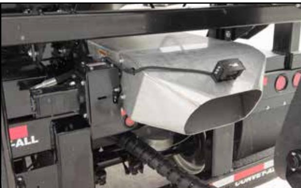
Fig 51 - Drive at underbin discharge
