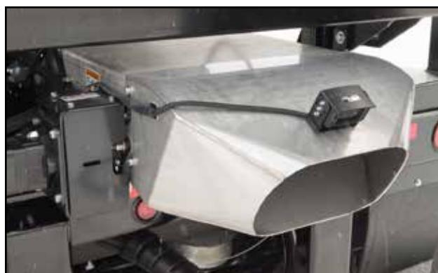
Fig 22 - Camera on underbin discharge
