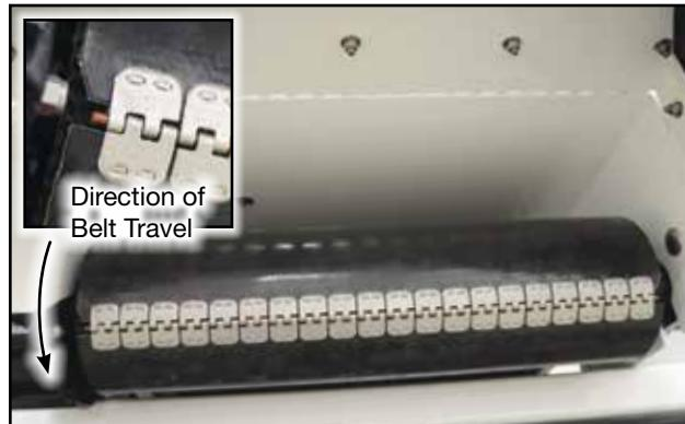
Fig 64 - Underbin conveyor belt lacing
