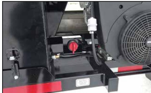
Fig 44 - Battery lock-out switch
