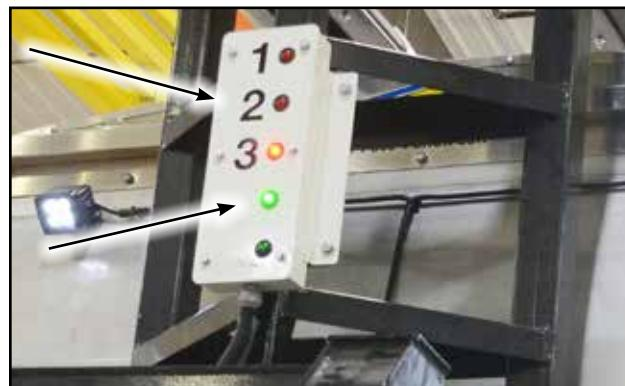
Fig 18 - Hopper gate status and swing centre LEDs
