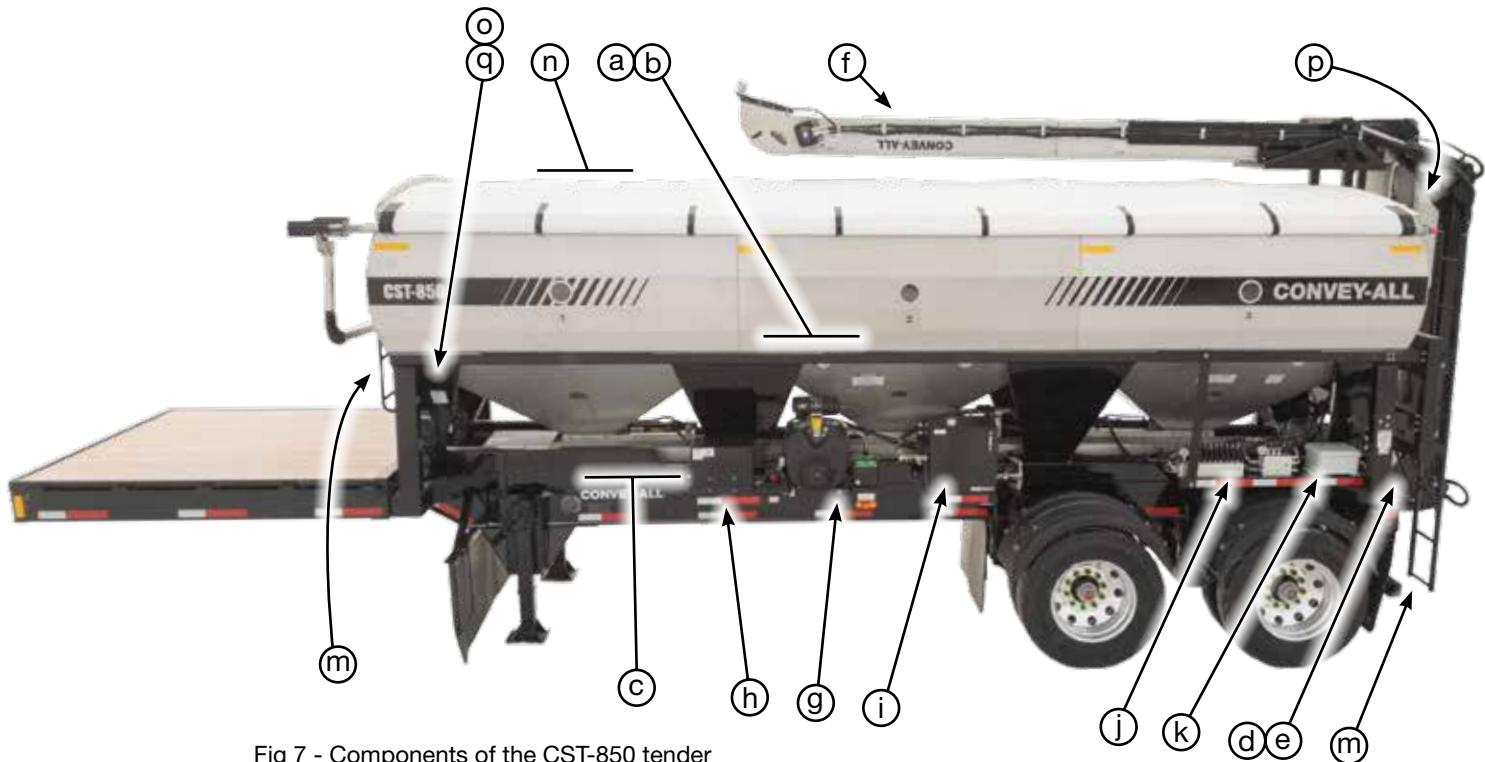
Fig 7 - Components of the CST-850 tender
