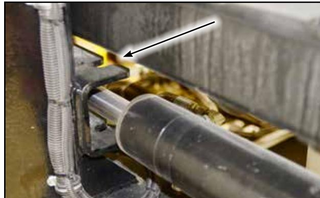
Fig 28 - Alternate cylinder frame connection
