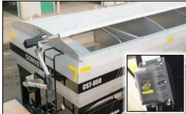
Fig 19 - Roll tarp and controls
