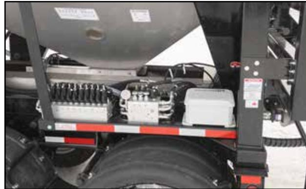
Fig 41 - Hydraulic valve bank
