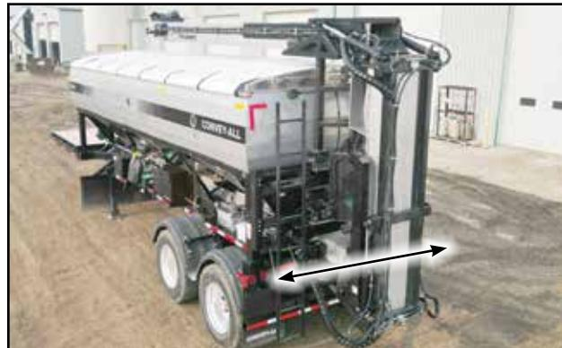
Fig 26 - Incline conveyor shuttle movement
