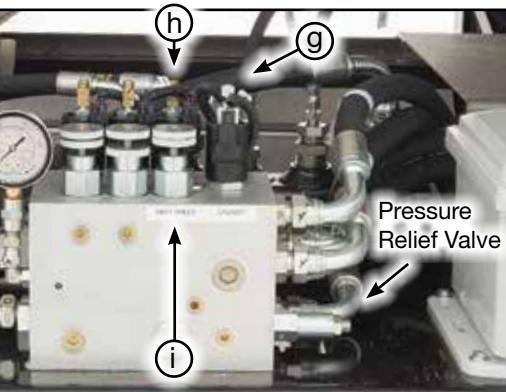
Fig 12 - Conveyor belt valve block
