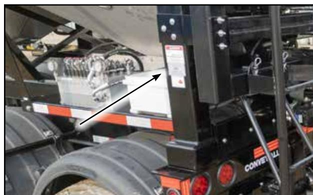
Fig 2 - Serial # on rear, corner, vertical support
