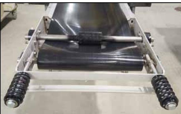
Fig 53 - Tension bolts. Underbin conveyor detail view
