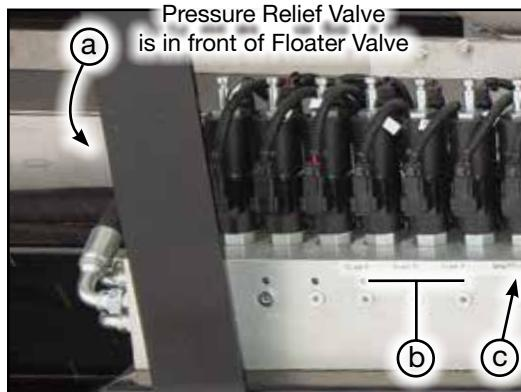
Fig 11 - Tender functions valve block
