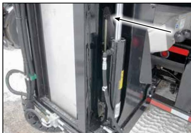
Fig 55 - Tension bolts inside incline conveyor frame
