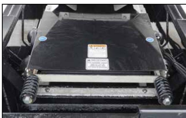
Fig 54 - Tension bolts on installed underbin conveyor
