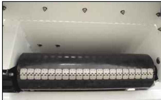
Fig 49 - Underbin conveyor belt lacing
