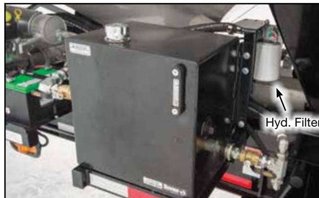
Fig 10 - Hydraulic oil reservoir and filter
